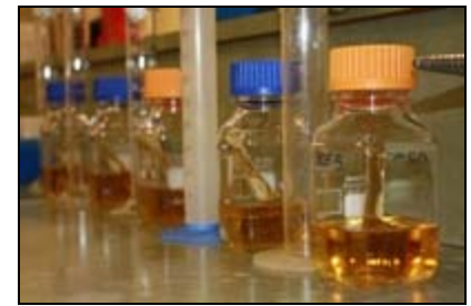
Media await the addition of water from ice samples for coliform analysis.
